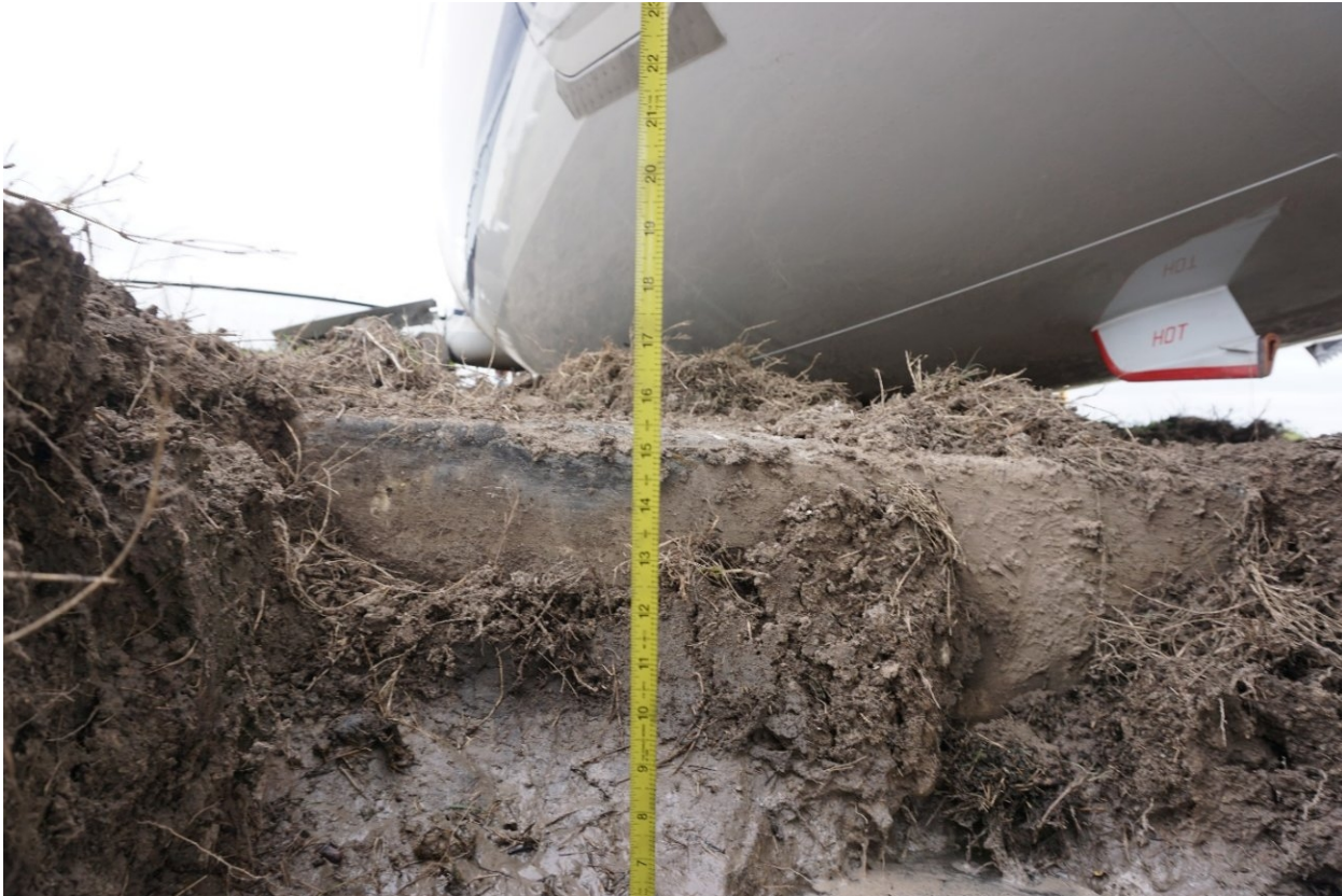
Figure 2. Photograph showing concrete “manhole” impacted by left main landing gear. (Source: Boeing.)
